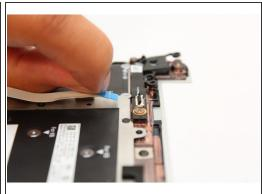
Disconnect the Fingerprint Cable from the Fingerprint Reader. Flip the black latch up using your fingernail or spudger end of the Framework Screwdriver and pull the cable straight out.
