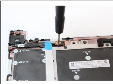
Using the PH0 bit in your Framework Screwdriver, screw the fastener into the Fingerprint Reader.
