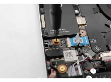
Using the T5 bit in the Framework Screwdriver screw in the two fasteners.
