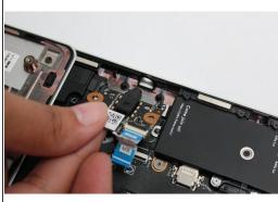
Place the Audio Board down by aligning the holes on the Audio Board with the alignment pins on the Bottom Cover and insert the headphone connector through the hole on the left hand side of the Bottom Cover.
