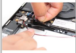
Locate one of two pieces of black tape and carefully peel it back to reveal the black and red speaker wires.
