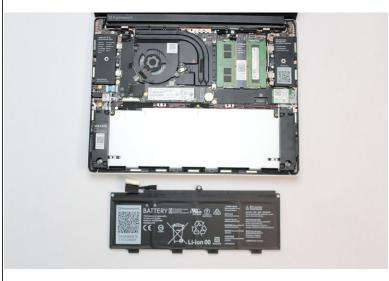
Use your fingernail to gently Lift the battery up and away from the bottom cover. Carefully lift it out and keep it in a safe place.
