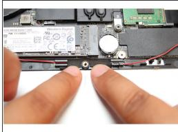
Place the wires into the wire router next to the other piece of black tape. Peel the tape back and place the wires under it. Cover the wires with same tape.
