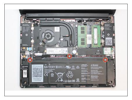
Using the T5 bit in the Framework Screwdriver, screw the three fasteners into place.
