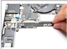
Peel the black tape back and place the wires under it. Cover the wires with same tape.
