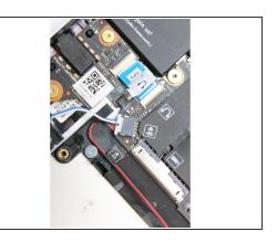
Using your fingers and a slight amount of force, insert the speaker connector straight into the Mainboard.
