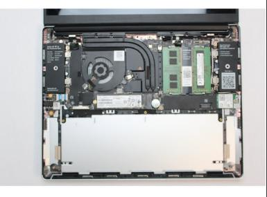
The speakers are now disconnected. You can lift both the left and right speaker out of the Bottom Cover.
