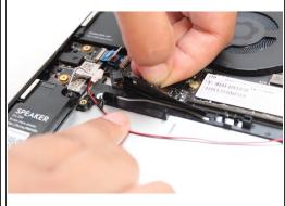
Locate one of two pieces of black tape and carefully peel it back to reveal the black and red speaker wires.
