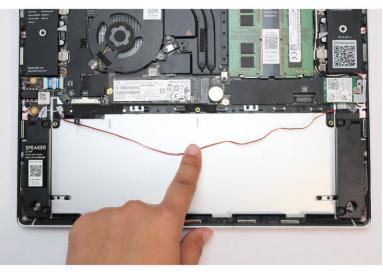
Carefully lift the wires out of the wire routers and very gently pull the wires down so that they are free.
