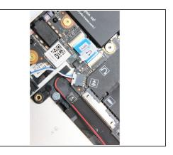
Using your fingers and a slight amount of force, insert the speaker connector straight into the Mainboard.
