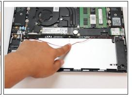
Locate the other piece of black tape and carefully peel it back to reveal the black and red speaker wires.
