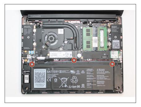
Using the T5 bit in the Framework Screwdriver, screw the three fasteners into place.
