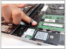
Using slight force, connect the Touchpad Cable by aligning it to the socket on Mainboard. You should hear it click into place once properly connected.
