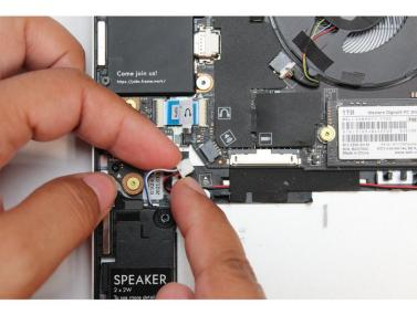
Using your fingernails disconnect the speaker connector from the Mainboard by gripping the edges
