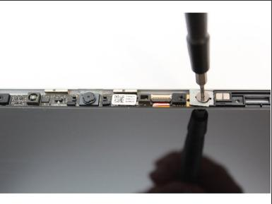
Using the T5 Bit in the Framework Screwdriver, unscrew the two fasteners connecting the Webcam Module to the Top Cover.
