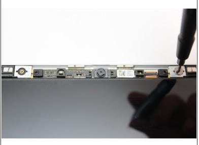
Using the T5 Bit in the Framework Screwdriver screw in both fasteners.
