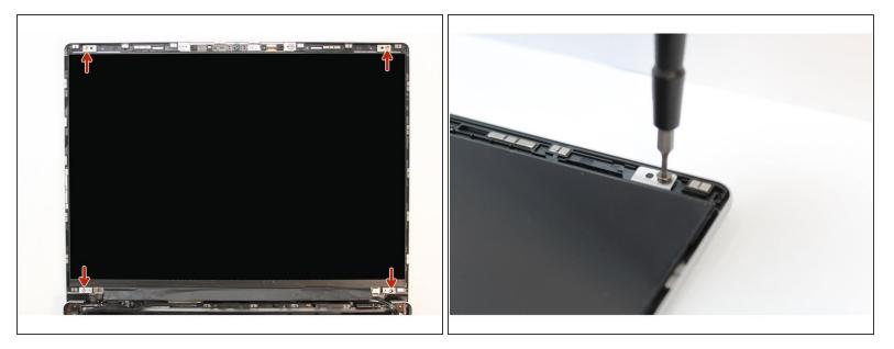
• Using the T5 bit in the Framework Screwdriver screw the four fasteners into place.
