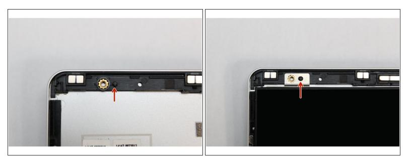
• There are four alignment pins located on the Top Cover. They are located right next to the four fastener slots. Place the silver brackets connected to Display directly over the pins.
