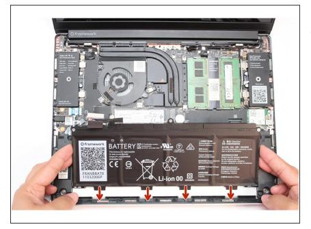
While handling the Framework battery with the plastic frame, slide it into the Bottom Cover. Use the first image as a reference.
