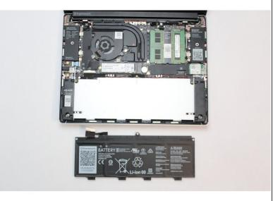
Use your finger tips to gently Lift the battery up and away from the bottom cover. Carefully lift it out and keep it in a safe place.
