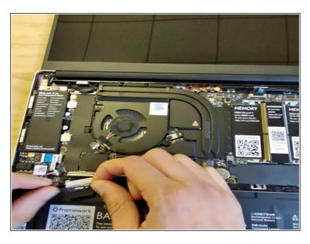
Carefully slide the Battery connector back into the mainboard, gripping both edges of the connector and sliding in straight without letting the connector twist or bend.
