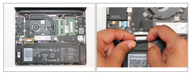
Be **extremely** careful when sliding the Battery connector out, as it is very easy to accidently bend the pins. Make sure to slide straight down, and avoid letting the connector twist or bend.
