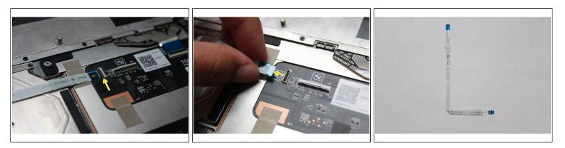
• Next, disconnect the Fingerprint Cable from the Touchpad Module. Lift the black latch up using your fingernail or spudger end of the Framework Screwdriver and pull the cable straight out.
