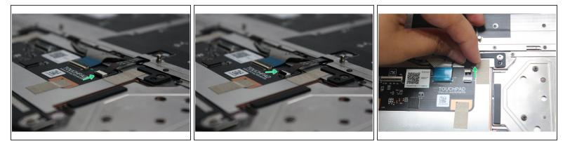
Using the spudger end of the Framework Screwdriver or your fingernail, disconnect the Keyboard Backlight cable from the Touchpad Module by switching the black latch up and sliding the cable straight out.
