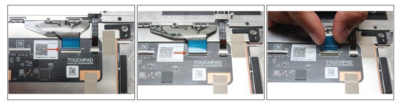
Using the spudger end of the Framework Screwdriver or your fingernail, disconnect the Keyboard Membrane from the Touchpad Module by switching the black latch up and sliding the cable straight out.
