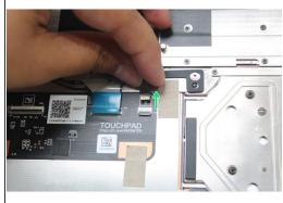
Using the spudger end of the Framework Screwdriver or your fingernail, disconnect the Keyboard Backlight cable from the Touchpad Module by switching the black latch up and sliding the cable straight out.
