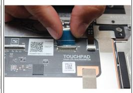
Using the spudger end of the Framework Screwdriver or your fingernail, disconnect the Keyboard Membrane from the Touchpad Module by switching the black latch up and sliding the cable straight out.
