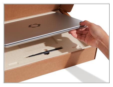
Locate the Framework Screwdriver in the package underneath the Framework Laptop and keep it handy - it's the only tool you'll need replace or upgrade any part of the product!
