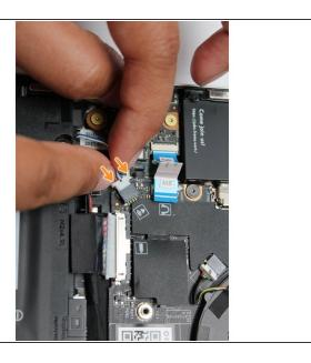
Using two fingers, slide the Speaker cable into the Mainboard using a straight motion and a slight amount of force.
