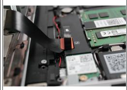
Using slight force, connect the Touchpad Cable by aligning it to the socket on Mainboard. You should hear it click into place once properly connected.
