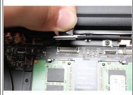
Using your fingers, carefully disconnect the Webcam cable on the top, right hand side by using the black pull tab to pull it directly upward.
