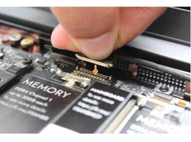
Hold the pull tab on the Webcam cable and connect it into the Mainboard by aligning the pins from the cable with the socket pins on the Mainboard.
