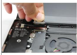
Using your fingers, carefully disconnect the Display cable on the top, left hand side by using the pull tab to pull it upward.
