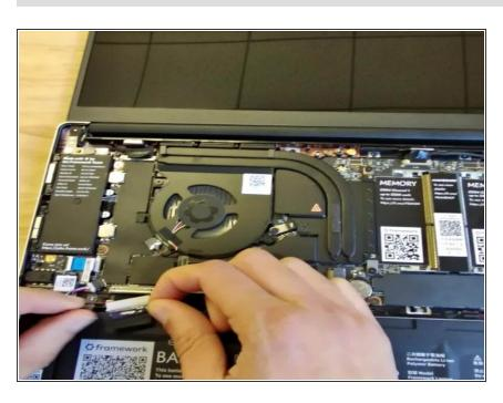
Carefully slide the Battery connector back into the mainboard, gripping both edges of the connector and sliding in straight without letting the connector twist or bend.
