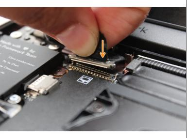
Hold the pull tab on the Display cable and connect it into the Mainboard by aligning the pins from the cable with the socket pins on the Mainboard.
