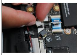
Using both fingers and a slight amount of force, disconnect the Speaker cable from the Mainboard by pulling it straight out.
