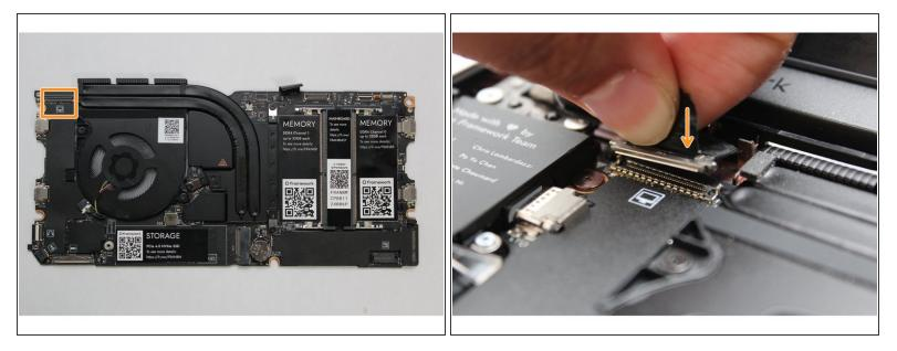
Hold the pull tab on the Display cable and connect it into the Mainboard by aligning the pins from the cable with the socket pins on the Mainboard.
