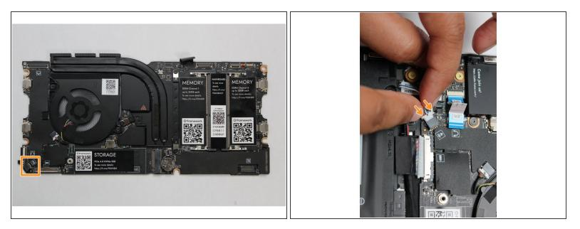
Using two fingers, slide the Speaker cable into the Mainboard using a straight motion and a slight amount of force.
