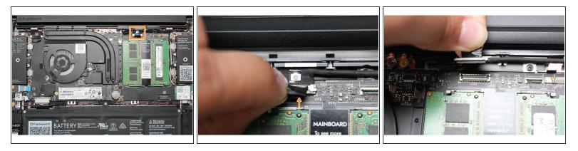
Using your fingers, carefully disconnect the Webcam cable on the top, right hand side by using the black pull tab to pull it directly upward.
