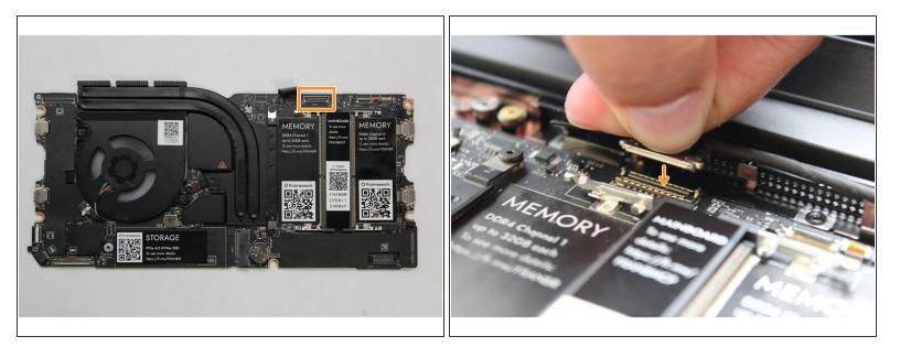
Hold the pull tab on the Webcam cable and connect it into the Mainboard by aligning the pins from the cable with the socket pins on the Mainboard.
