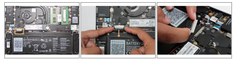
Gently disconnect the Battery by gripping the connector edges with both fingers and slide the connector away from the socket.
