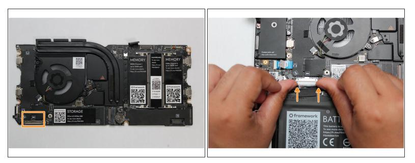
Plug the battery into the Mainboard using two fingers so that you can slide the connector into the socket with an even, straight motion.
