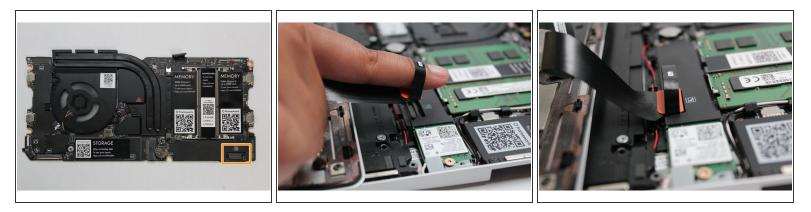
Using slight force, connect the Touchpad Cable by aligning it to the socket on Mainboard. You should hear it click into place once properly connected.
