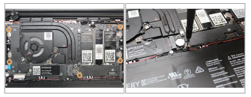
Using the T5 bit in the Framework Screwdriver, unscrew the five fasteners holding down the Mainboard.
