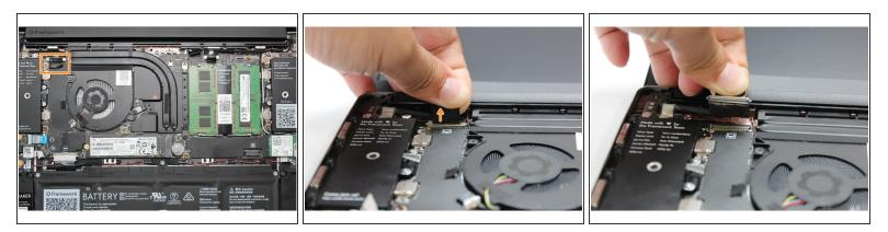
Using your fingers, carefully disconnect the Display cable on the top, left hand side by using the pull tab to pull it upward.
