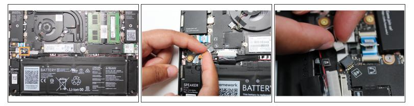
Using both fingers and a slight amount of force, disconnect the Speaker cable from the Mainboard by pulling it straight out.
