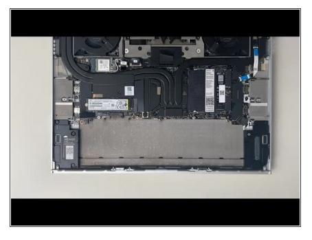
Lower the Battery into place, first aligning the bottom of Battery in the bottom cover as shown, then push
