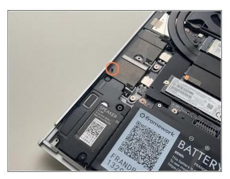
Place the Mid Plate back onto the system, aligning the holes in the Mid Plate with the two guide posts.
