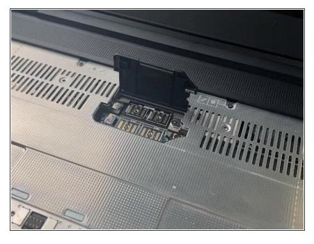
With the Interposer removed, loosen the 2 captive fasteners holding the Graphics Module in place.
