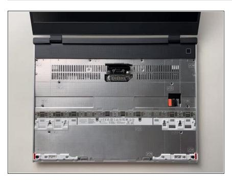
Tighten the 2 captive fasteners to secure the Expansion Bay Shell in place.
