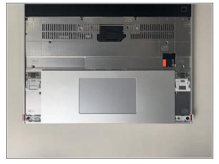
• After removing the Spacers, the Touchpad module can be removed in the same way. Gently slide it downwards from both sides and then lift away as shown.
