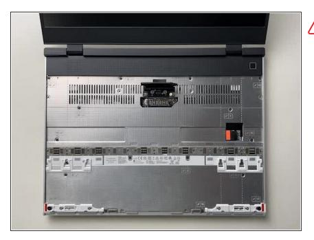
A Before closing the lid of the Laptop to remove or swap the Expansion Bay module, make sure the Interposer Door is closed.
