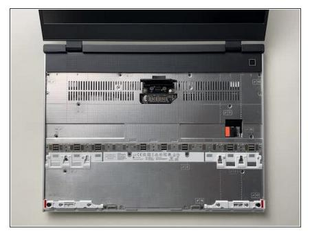
With the Interposer installed, close the Interposer Door.
