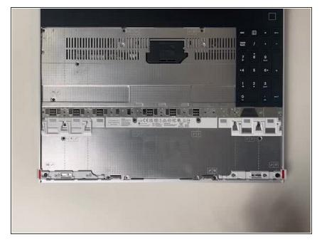
Remove your Input Modules or Spacers in the same way as the Keyboard, lifting from the bottom using the pull tabs as shown.
