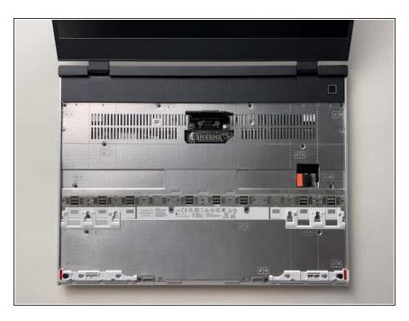
Tighten the 2 captive fasteners to secure the Graphics Module in place.
