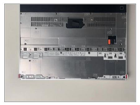
Using the pull tab, gently press the Mid Plate connector down to connect it to the Mainboard.
