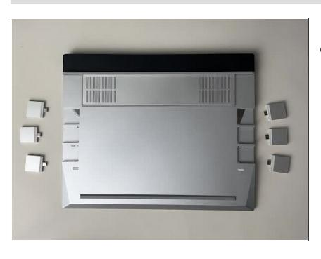
Before inserting Expansion Cards, make sure that the Expansion Card Latches are open, these will appear red/orange when open and light grey when closed.
