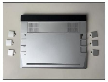
Before inserting Expansion Cards, make sure that the Expansion Card Latches are open, these will appear red/orange when open and light grey when closed.
