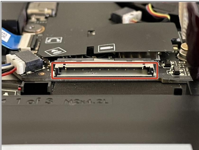
⚠ Before plugging the Battery connector back in, double check the pins on the Battery receptacle on the Mainboard, and make sure none of them look bent.
