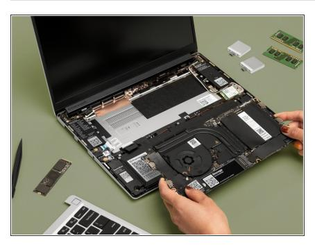
Before soldering, you should remove the Mainboard from the system, following the <u>Mainboard guide</u> up to Step 16.
