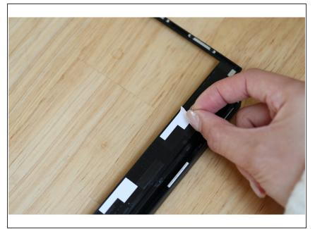
• If installing a new Bezel, remove the liner pieces on the bottom of the Bezel to expose the adhesive.
