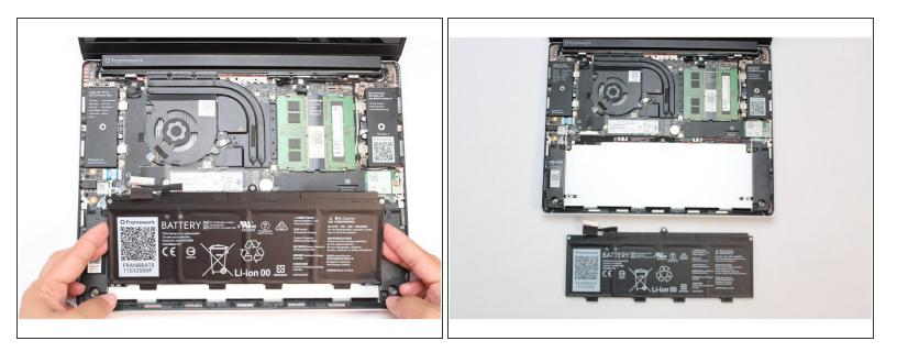
Use your finger tips to gently Lift the battery up and away from the bottom cover. Carefully lift it out and keep it in a safe place.
