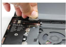
Using your fingers, carefully disconnect the Display cable on the top, left hand side by using the pull tab to pull it upward.
