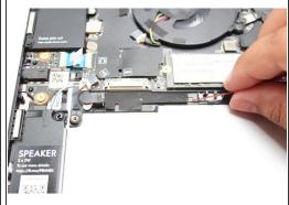
Peel the black tape back and place the wires under it. Cover the wires with same tape.
