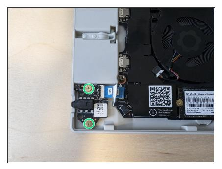
Using two of the three included PCB fasteners, install the Audio Board in the lower left of the case.
