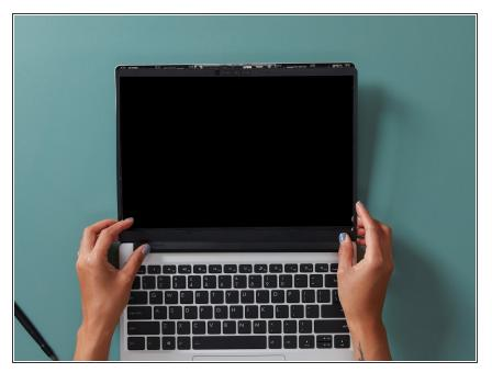
Now that all the cables that route through the hinges are re-installed, it's time to install the Bezel. Align the corners of the Bezel to the display and place it down. The Bezel is attached by magnets and should easily click into place.
