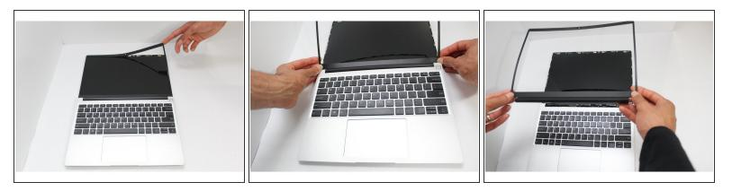
• Open the Framework Laptop 180 degrees to remove the Bezel.
