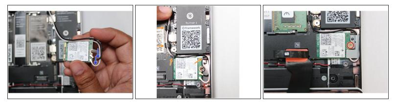
• Carefully connect the black and white WiFi antenna cables into their respective sockets on the module. Make sure to align them well before applying force to click them into place, as the connectors are small and fragile.
