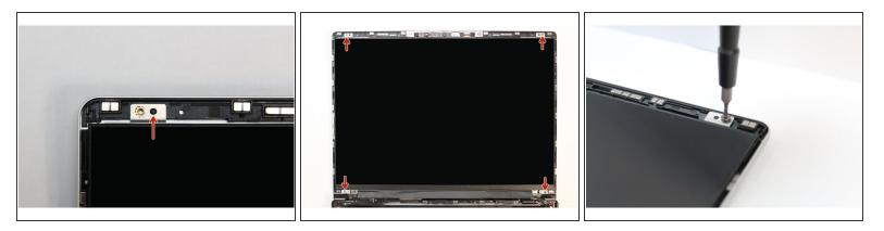
• There are four alignment pins located on the Top Cover. They are located right next to the four fastener slots. Place the silver brackets connected to Display directly over the pins.
