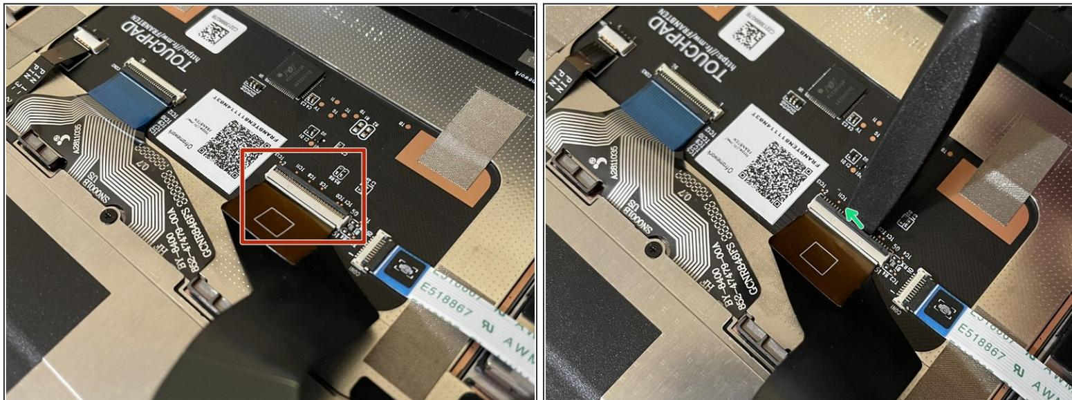
**⚠ Before closing up the laptop, make sure that the Touchpad end of the Touchpad Cable is fully seated in the receptacle.**
