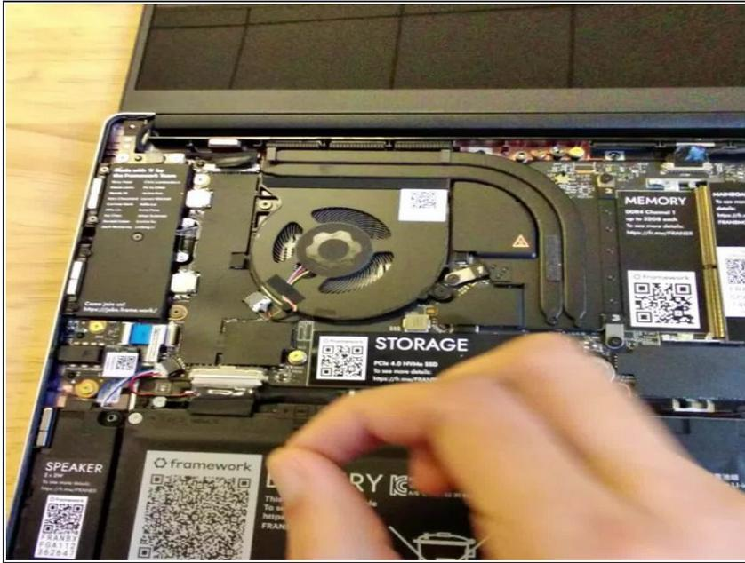
⚠ Be **extremely** careful when sliding the Battery connector out, as it is very easy to accidentally bend the pins. Make sure to slide straight down, and avoid letting the connector twist or bend.
