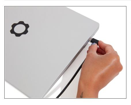
Plug your Power Adapter back in and let the laptop charge for 24 hours. You can use your laptop during this time, but keep it plugged in to let the RTC Coin Cell fully recharge. If you run into any issues during this process, please <u>reach out to the Framework Support team</u>. We're here to help.
