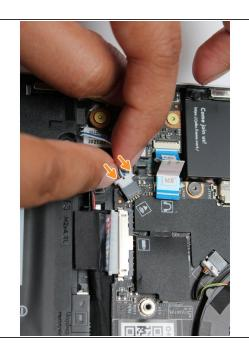
Using two fingers, slide the Speaker cable into the Mainboard using a straight motion and a slight amount of force.
