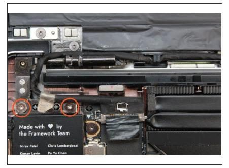
Using the T5 bit in the Framework screwdriver, the two fasteners on the left and right Hinges connecting to the Bottom Cover will need to be un-fastened.
