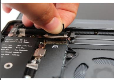
Hold the pull tab on the Display cable and connect it into the Mainboard by aligning the pins from the cable with the socket pins on the Mainboard.
