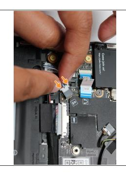
Using two fingers, slide the Speaker cable into the Mainboard using a straight motion and a slight amount of force.
