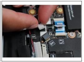
Using both fingers and a slight amount of force, disconnect the Speaker cable from the Mainboard by pulling it straight out.
