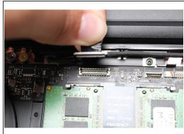
Using your fingers, carefully disconnect the Webcam cable on the top, right hand side by using the black pull tab to pull it directly upward.
