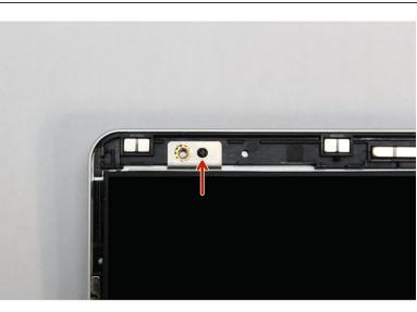
There are four alignment pins located on the Top Cover. They are located right next to the four fastener slots. Place the silver brackets connected to Display directly over the pins.
