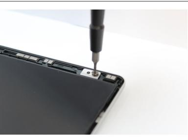
Using the T5 bit in the Framework Screwdriver screw the four fasteners into place.
