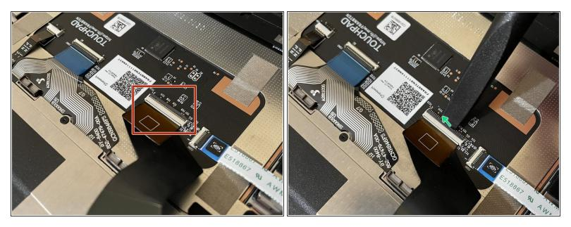
A Before closing up the laptop, make sure that the Touchpad end of the Touchpad Cable is fully seated in the receptacle.
